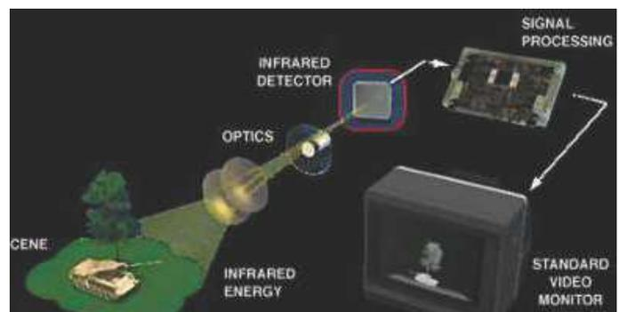
[The basic components of a thermal-imaging system]
