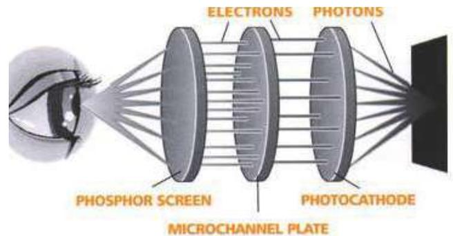
[The image intensifier tube changes photons to electrons and then back again]
